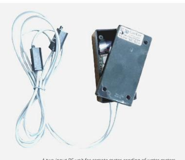
A two input RF unit for remote meter-reading of water meters.
