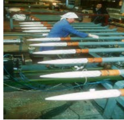
Manufacturing of hail damage repelling rockets filled with silver-iodide in Russia.
