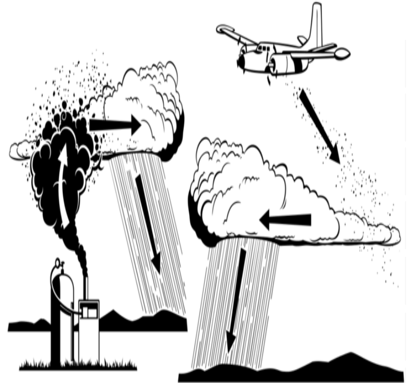
The two basic ways for hail damage prevention: the dangerous clouds must be attacked from above and / or from below.
