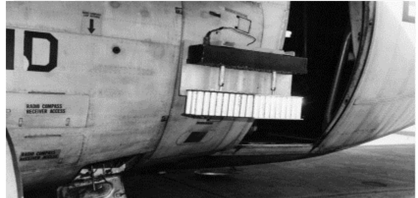
Rain making equipment on the US Air Force's WC-130E transport aircraft used in Vietnam
