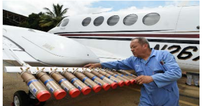
A silver-iodide, sodium-chloride and calcium-chloride dosing unit is being fixed on the wings of a plain in India.
